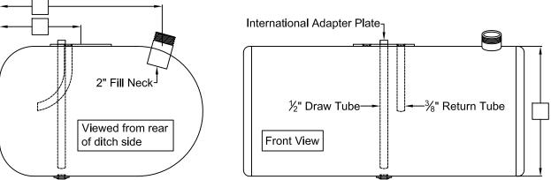
Please note: All sizes are NPTF unless otherwise noted and reference all measurements from the lateral weld seam and the end cap weld seam to the center of the fittings.
